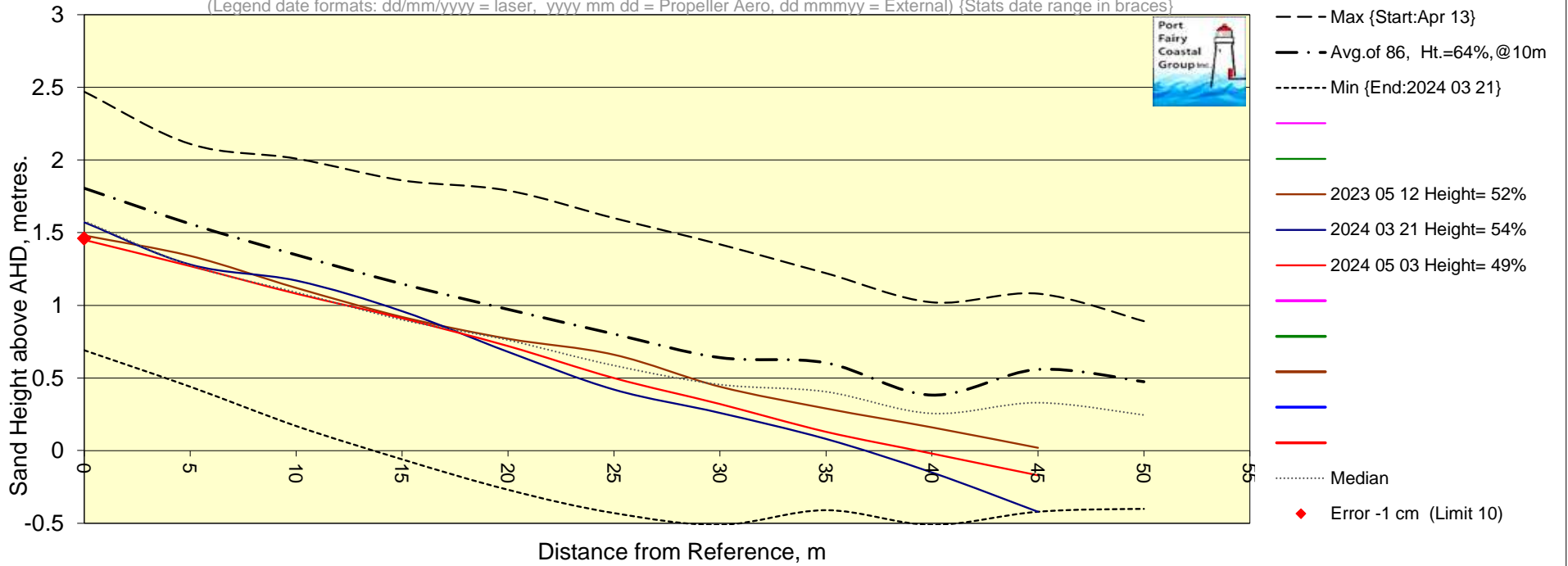
Chart PFETP3 Post 3 Transverse Profile perpendicular to dune scarp.
